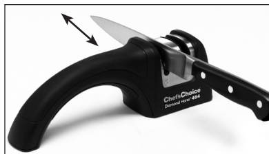
Figure 1. Knife in Stage 1. Use back and forth sharpening strokes with modest downward pressure (See text.)
